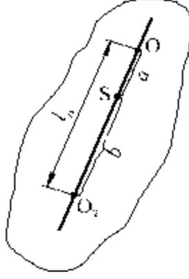
Figure 1: Physical pendulum with two suspension points.
