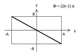
The transition from one figure to another can be realized by moving the microphone with respect to the speaker, which results in the phase shift  $\Phi = \pi$ . The minimal distance between the positions corresponding to both figures is D, which is related to the wave period T, the wavelength  $\lambda$  and the frequency f by means of the formula:
