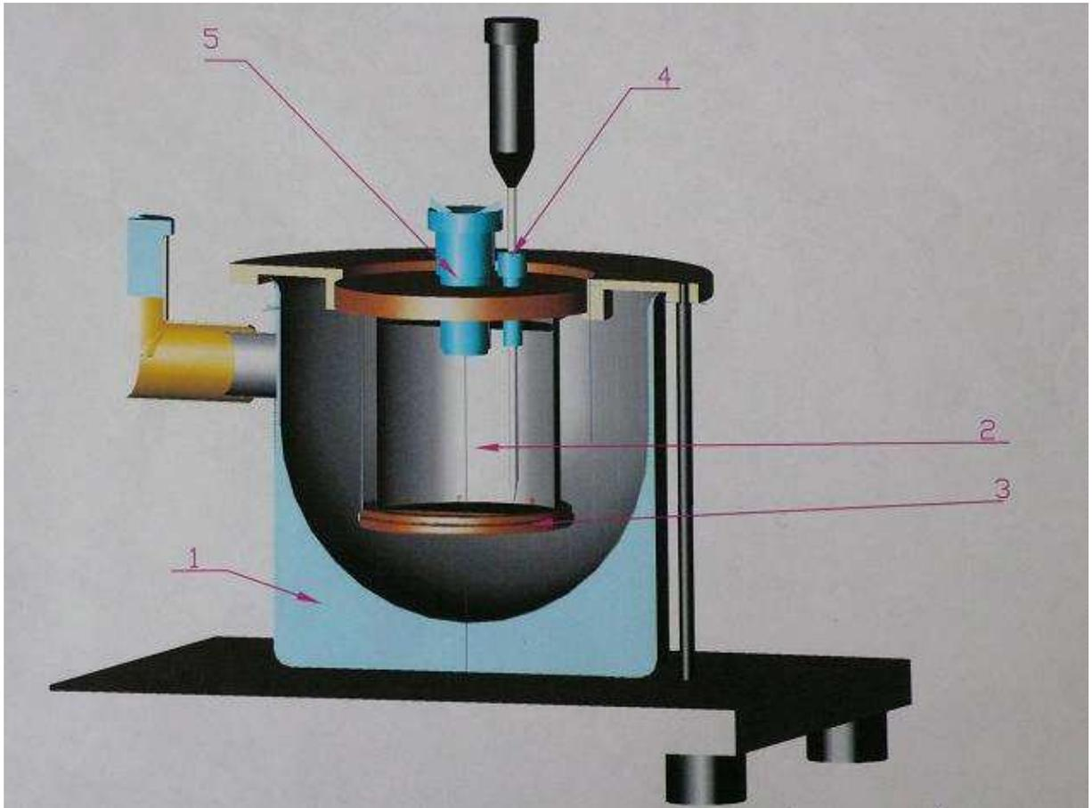
Figure 1: A water jacket calorimeter
