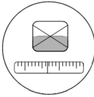
Fig.1. View through the eyepiece of a correctly adjusted refractometer.
