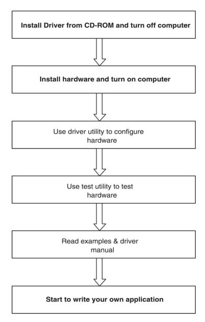
Figure 1.1: Installation Flow Chart
