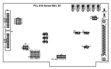
Figure D.1: PCL-818HD/HG/L VR Assignment
