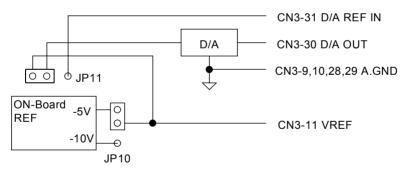
Figure 3.2: Analog Output Connections
