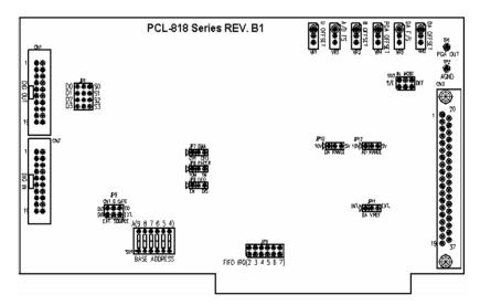
Figure 3.1: Connectors, Jumpers & Switches
