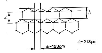
Fig.3. Graphite planes for first two interference rings
