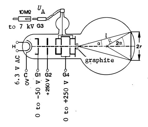
Fig.1. Electron diffraction vacuum tube
