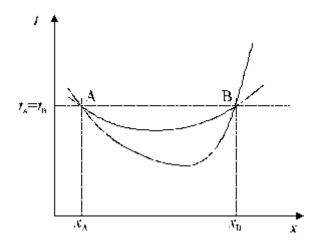
Figure 4: Plot of relation T(x) for the pendulum suspended from both axes. Horizontal coordinates of the cross-section points fulfil the conditions:  $T_A = T_1(x_A) = T_2(x_A)$ ,  $T_B = T_1(x_B) = T_2(x_B)$ .
