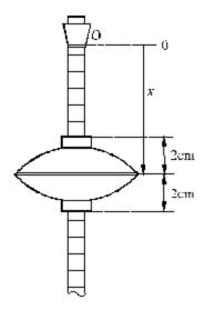
Figure 3: Illustration of measurements of distance x between movable mass R and axisO<sub>1</sub>.
