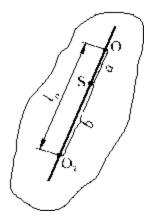
Figure 1: Physical pendulum with two suspension points.
