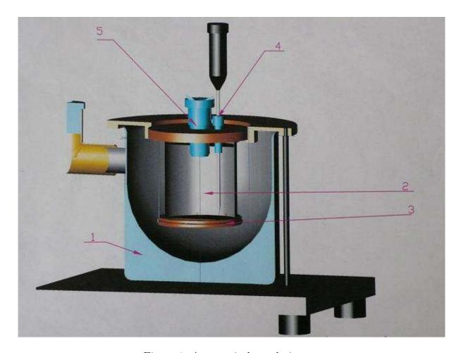
Figure 1: A water jacket calorimeter
