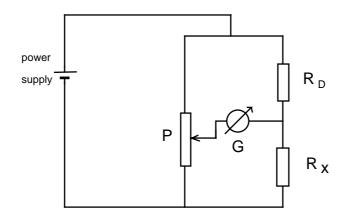
Figure 1. Experimental circuit
