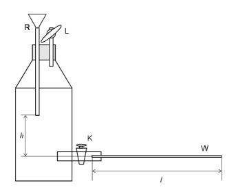
Fig. 1. Scheme of the experimental setup for the measurement of the viscosity coefficient of water
